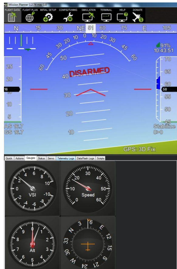
Fig.8. Screenshot of HUD on ground control Station
