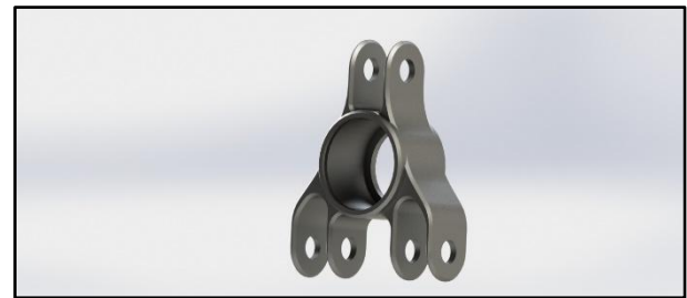
Fig 11: Rear upright modeled in SolidWorks.
