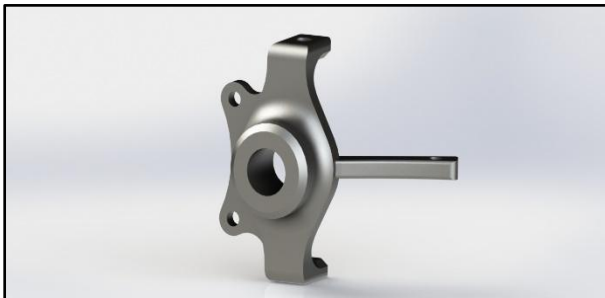
Fig 8: Front upright modeled in SolidWorks.
